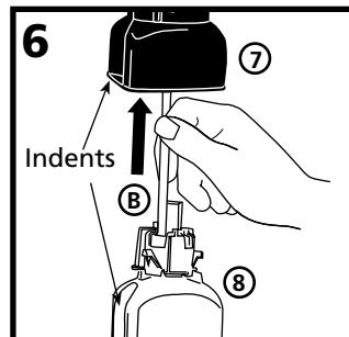
Feed the dispense tube (B) on the refill bottle (8) through the bottle support (7), aligning the two indents. Slide the refill upward until it snaps into place.
