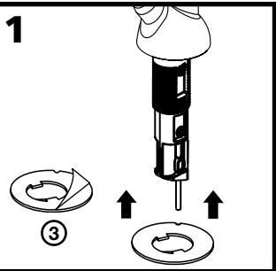
Locate the adhesive gasket (3). Remove the liner from the top of the adhesive gasket and affix to the bottom of the dispenser. Remove the liner from the bottom of the gasket.
