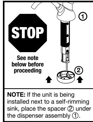
**NOTE:** If the unit is being installed next to a self-rimming sink, place the spacer (2) under the dispenser assembly (1).
