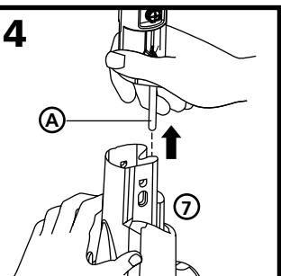
Align the metal rod (A) from threaded shank with small guide hole in the bottle support(7). Slide the bottle support up onto the rod.
