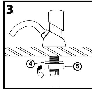
From underneath the counter, secure lock washer (4) and mounting nut (5) and tighten to underside of counter.
